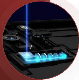
Multi-Camera Combo, Folded optics (WFOV -> 50x Super Zoom)
