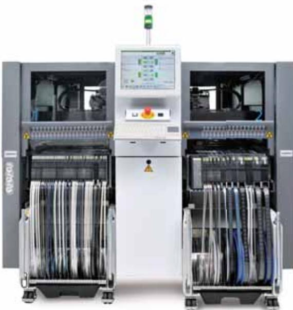
The ability of SIPLACE SX to handle very tiny components (01005) makes it an ideal solution for the assembly of smartphones
